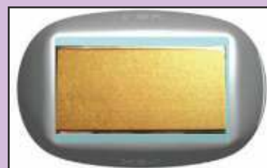
Fig 4 : View of X6-1 transducer, looking at the face of the transducer with the lens removed. The 2D array with 9212 active elements is visible.
